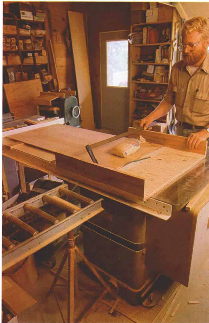
The basic sliding table (photo above) makes crosscutting easy on the table saw. Here it is being used to trim the end of a glued-up oak panel. The bag of lead shot on the workpiece helps to hold it in place. Note the scrap stock "crutch" beneath the end of the workpiece; it compensates for the thickness of the sliding table.
