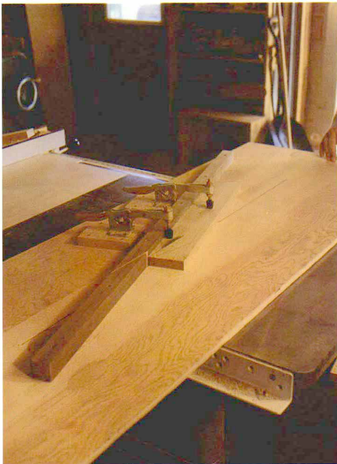
The author's "board stretcher" is a simple sliding saw table used to cut scarf joints (photo above).
