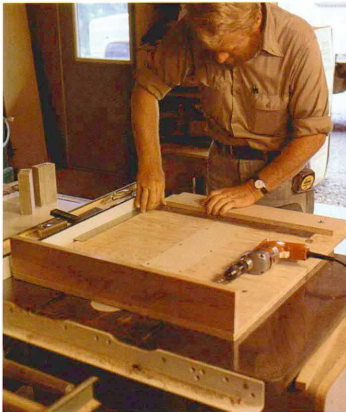
To provide an accurate guide against which the permanent fence can be registered, a temporary fence (photo above) is first screwed to the sliding table. It can be adjusted into precise position with a framing square held against the saw's rip fence. Wood guides beneath the sliding table are just visible in this photo.
